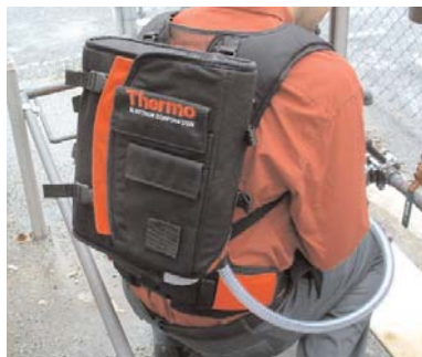
Analyzer bag protects TVA1000 and may be used with standard shoulder strap or optional framed backpack
