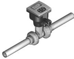
The compact mounting kit F9.KC1 includes the compact plastic adapter with gasket for IP65 watertight installation, the compact cap, the locking ring and four fixing screws for mounting the monitor directly onto the sensor. The instrument and the kit can be ordered separately (code F9.20 for the monitor and code F9.KC1 for the kit) or together using the code F9.20.XX.
