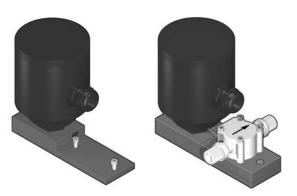
This Kit consists of an additional IP65 housing mounted aside the sensor via a PVC plate. It is a blind transmitter designed to convert the signal from the sensor into a 4-20 mA output for long distance transmission.
